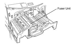
Print problems such as soiling of the reverse side of printed pages may occur if the paper feed unit becomes dirty. Clean the paper feed unit according to the following procedure.
